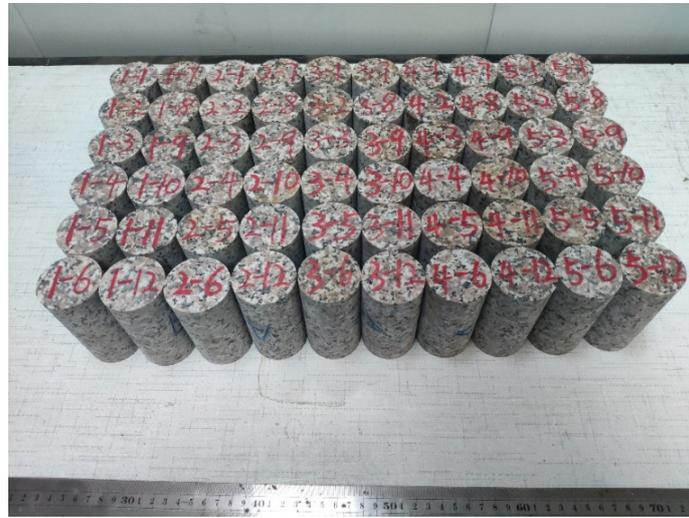
Fig. 1. Granite specimens
